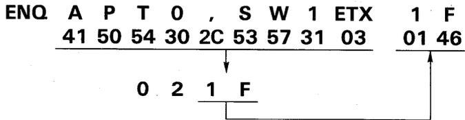
EXAMPLE: All slave units (when sending information to turn the #2 OUTPUT to "ON").
