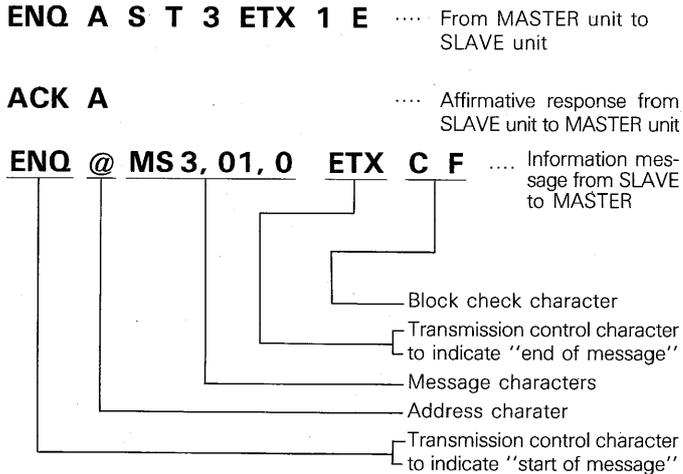
The contents of the message sent from the SLAVE to the MASTER indicate that the SLAVE unit being controlled under ADDRESS NO. 1 is a PWR18-1. 8Q.
