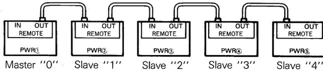
Up to 5 machines of the same model can be connected. If more than 5 machines are connected, control may become impossible to achieve.
