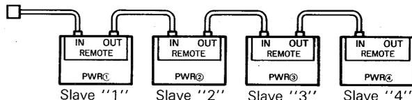
Unlike in MASTER operation, machines of different types can be connected. However, the maximum number of machines connected should be limited to four.
