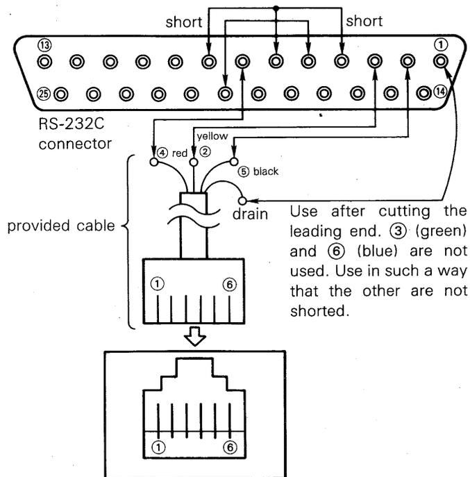
Use IN remote terminals ②~⑥ and OUT terminals ③, ④ floated from the remote IN ① and OUT ① terminals (from the frame GND terminals on the master and Slave units). Without this procedure, the PWR may not function correctly.
